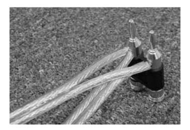
Loosely twist the "+" wires from each subwoofer (or tower base) together, then repeat for the "-" wires. Loosen the red and black thumbscrews on the Adapter until the hole in the shaft is fully revealed. Insert the twisted pair of "+" speaker wire to the hole marked with red. Tighten until the wire is securely clamped. Repeat the procedure for the "-" speaker wire and black thumbscrew. The Adapter can now be inserted into the A1 amplifier's "speaker out" terminal posts.
